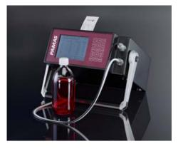
The PAMAS S40 portable particle counter analyses oil, fuel or phosphate-ester. The instrument is calibrated according to ISO 4402 and/or ISO 11171.
